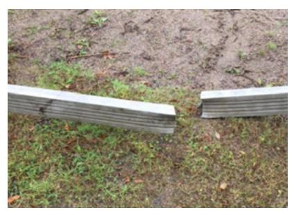
"Always place your straps around both front legs. Placing a single strap in the middle of the front frame will result in this breakage"
